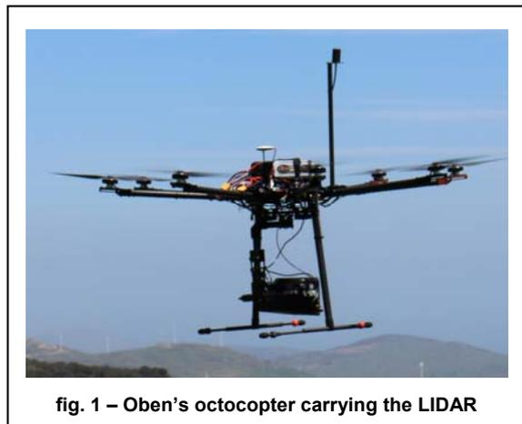
fig. 1 – Oben’s octocopter carrying the LIDAR
